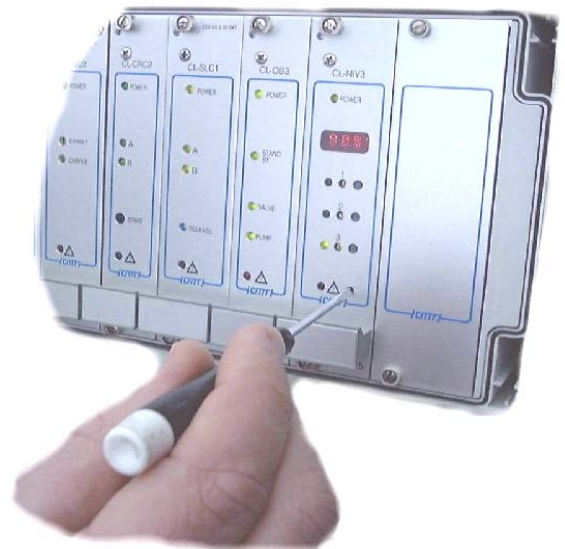
FIG. 5 Setting the CAL-level
