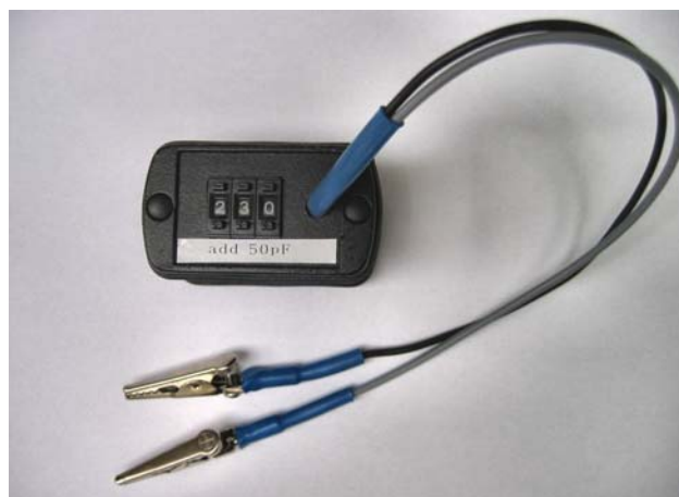
Fig.7 directly adjustable three-digit capacity simulator.
