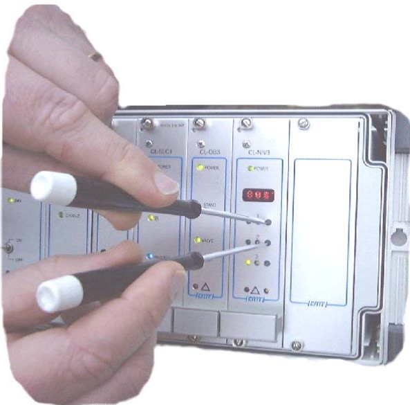
FIG. 4 Pushing 1 and 2 so the CAL-level can be set
